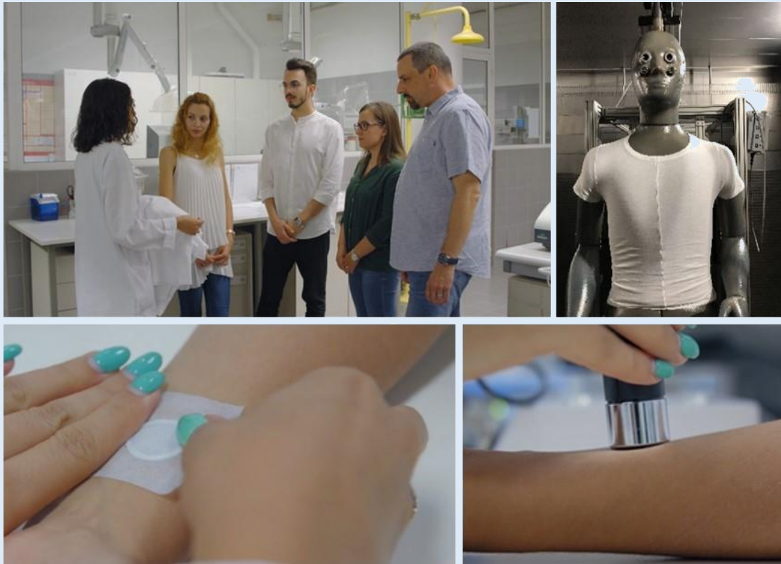
Figure 6. In-vivo and in-vitro evaluations of the performance (above) and the safety (below) of skin thermal comfort demonstrators.
